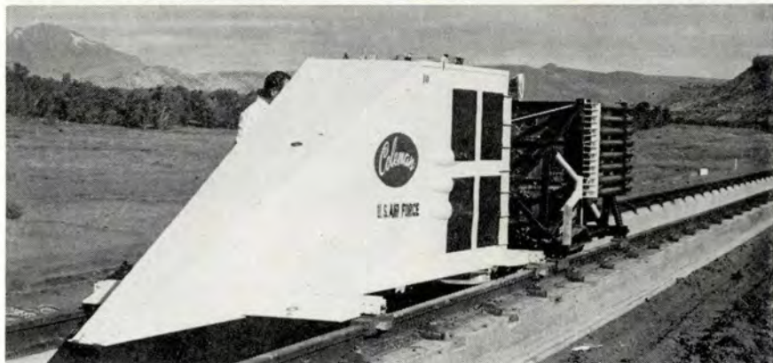
Left. The Hurricane Mesa supersonic track is shown in part, looking to the North. Above. A rear view of test vehicle used in tests of one upward ejection seat, F-102 configuration. Below, The Standard Hurricane Supersonic Research Site test sled and 5KS rocket propulsion vehicle.
