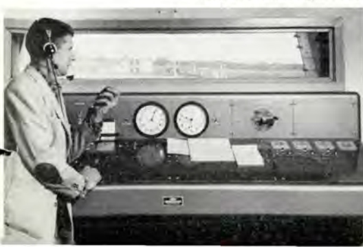
Firing Control Console with mirror image of sled; the oscillo-camera and operator; data room with 7 channel tape recorder for storing information from sled and dummy during run and ejection.
