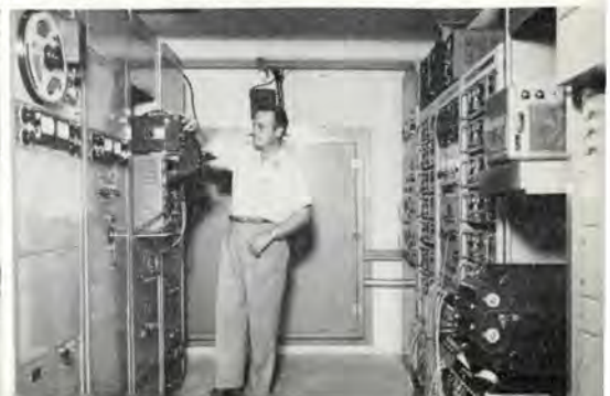
Firing Control Console with mirror image of sled; the oscillo-camera and operator; data room with 7 channel tape recorder for storing information from sled and dummy during run and ejection.
